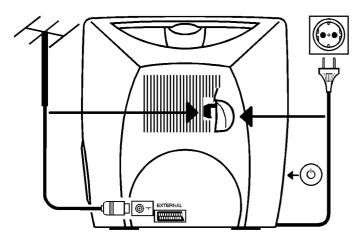
1 Insert the aerial plug into the \\_\_\_ socket.
